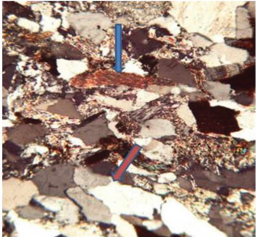
Figure 7. Photomicrograph of rock sample McD-3, collected near well Mcd-0203, in the Elkhorn area, McDowell County, West Virginia. [Abundant quartz grains exhibiting sutured grain boundaries (red arrows). Highly birefringent phyllosilicate grains fill all available pore spaces. Field of view approximately 1.1 mm.]
